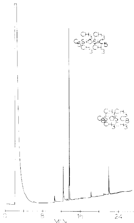
Fig. 2. Direct analysis by capillary GC of the acid hydrolysis products of a dimethyloctyl 10- \mu m silica phase, using C 5 dimer as an internal standard. The smaller unidentified peaks were from the internal standard and from slight impurities in the hexane extractant. GC conditions: column, SGE BP-1; split injection; temperature, from 100 to 250°C at 8°C/min. Other instrumental and reaction conditions are described in the Experimental section.
